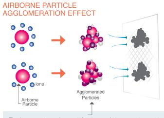
The ions attach to the particle, the particle grows larger by attracting nearby particles of the opposite polarity, thereby increasing the filtration effectiveness, or falls to the ground and out of breathing zone.
